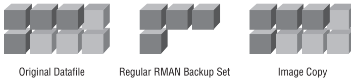
FIGURE 3.3 Image vs. regular backups
