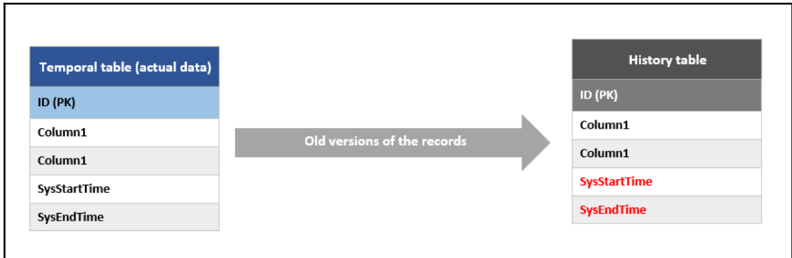
Figure 12-1. How system-versioning works
