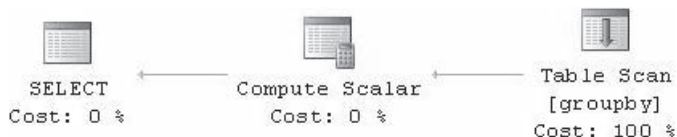
FIGURE 8-4 Query plan with aggregate operation removed
