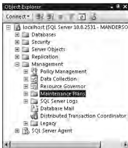
Figure 10-27 Maintenance Plans located under the Management node
