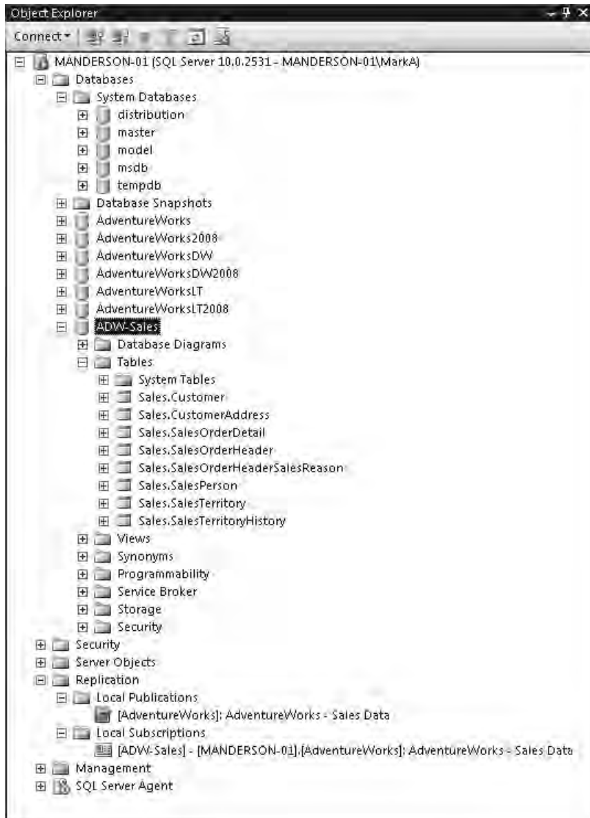
Figure 11-49 Replication management in SSMS
