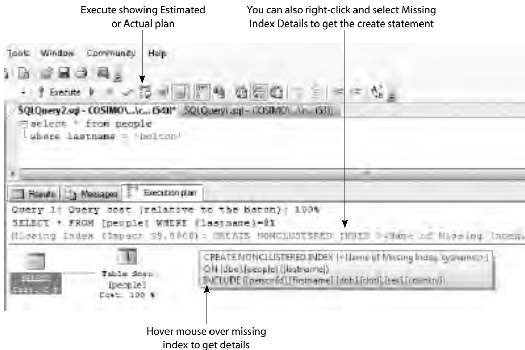
Figure 8-11 Missing-index details in an execution plan
