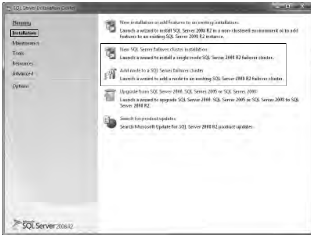
Figure 9-7 Integrated cluster installation and “add node” function
