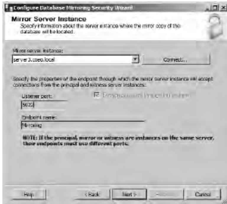
Figure 9-14 Connecting to the mirror server
