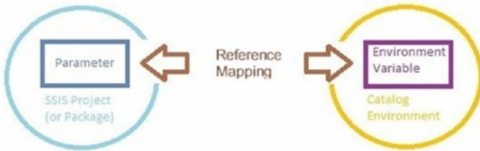
Figure 5-12. A reference mapping between an SSIS catalog project parameter and an SSIS catalog environment variable
