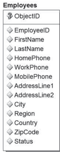
FIGURE 7.8 The Employees entity for Mountain View Music, with primary keys and all attributes added
